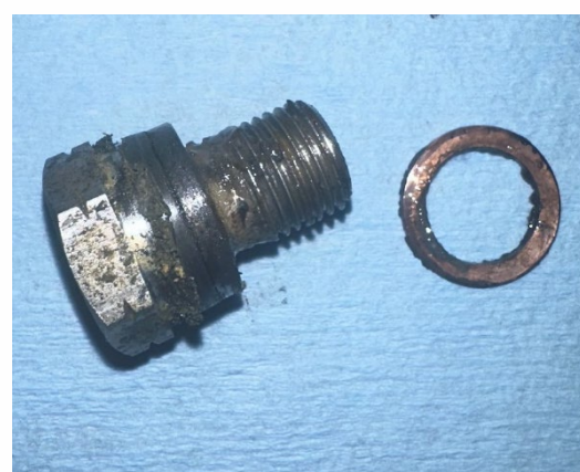
Tail plug elastomer failure/intrusion of well solids
