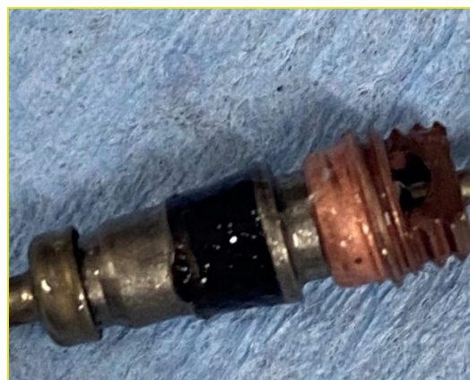
Valve core elastomer degradation/deformity
