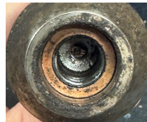
Intrusion of well solids into dome cap bore
