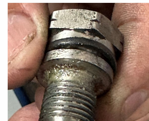
Tail plug elastomer degradation/failure
