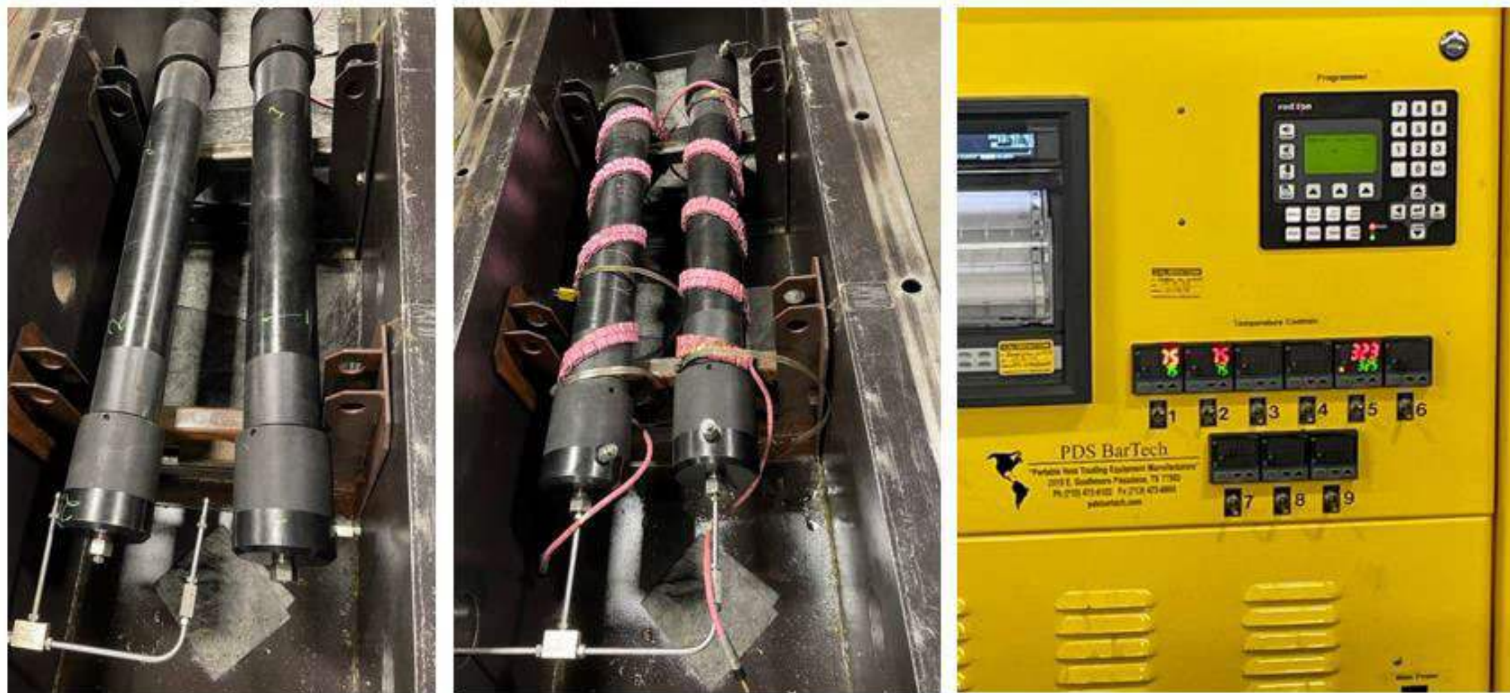
VALVES BEING LOADED INTO TESTING CHAMBERS AND PRESSURE BUNKER WITH HEAT COILS AFFIXED
