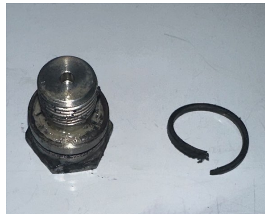
Tail plug elastomer degradation/failure
