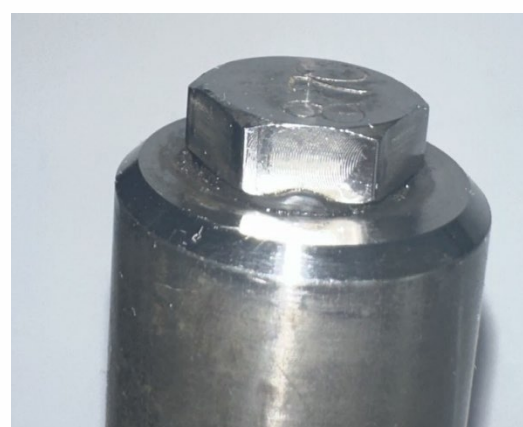
Tail plug elastomer extrusion
