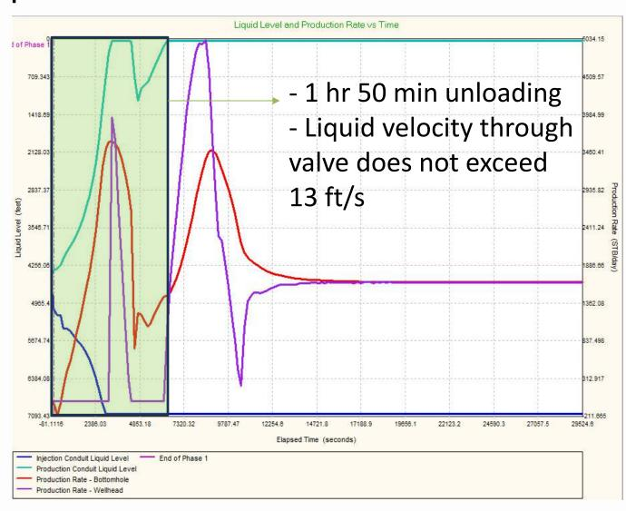
Regular unloading procedure durations are 3x higher in practice. Fast unloading durations in practice generally match simulated times.
