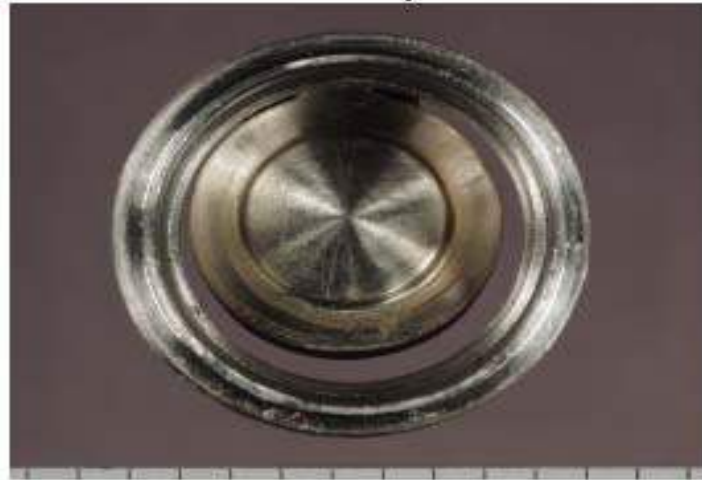
Flapper of HRO w/ 1/8" with a slight mark caused by sliding of flow tube. The mark is inner side of flapper.
