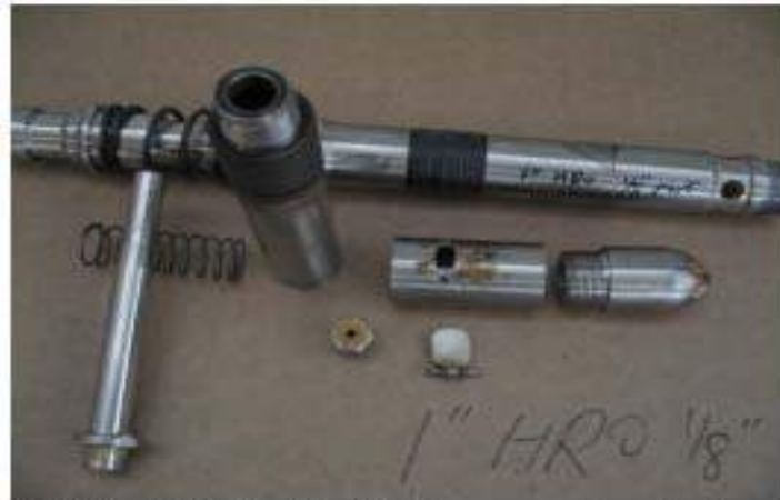
HRO w/ 1/8" after 7 days erosion test
