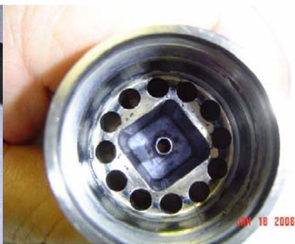
Photo 4.0 (Nozzle ID after 800 bbl liquid flow test)
