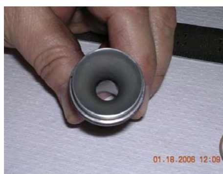
Photo 7.0 (Venturi Orifice after 800 bbl liquid flow test)
