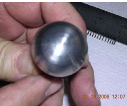
Photo 3.0 (Dart after 800 bbl liquid flow test)
