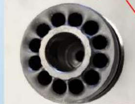
Valve Housing Eroded
