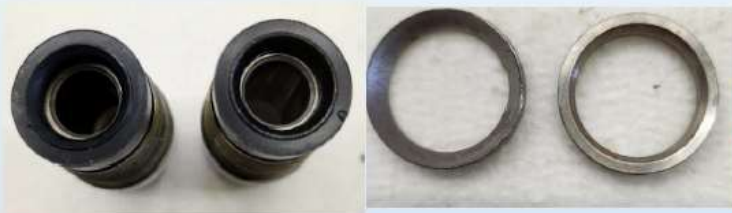
Seal Pad and Washer Worn After 400 BBL
