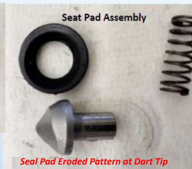
Seal Pad Eroded Pattern at Dart Tip
