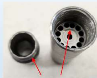
Valve Housing Eroded
