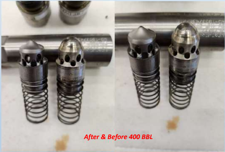
Seal Pad and Washer Worn After 400 BBL
