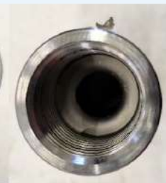
Polished Opening Eroded ~0.156"
