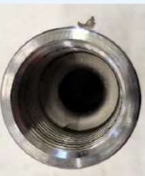
Polished Opening Eroded ~0.156"
