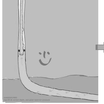
Gas lift mandrel(s) are placed at optimum depth when the well is completed, based on a reservoir pressure that can efficiently deliver fluids to the gas lift valve(s) HANSENPUMPS
