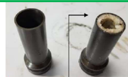
Scale deposition had completely blocked the component
