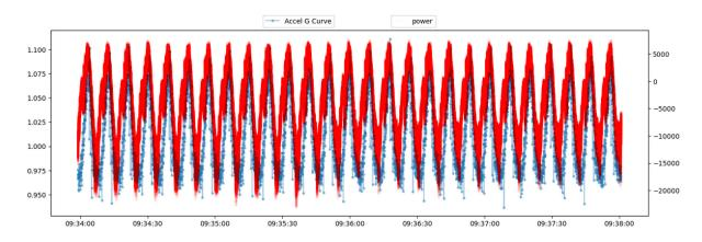
The plot above was created without downsampling. Since SAM4 is sampled at 20 kHz, the red curve consists of nearly 5 million points being plotted across 4 minutes. This amount of plotting points is clearly overkill. The plot below shows the same information, but with SAM4 data downsampled at 30 Hz. The conclusion is still the same: blue and red peaks align perfectly (up to a margin of synchronisation error).
