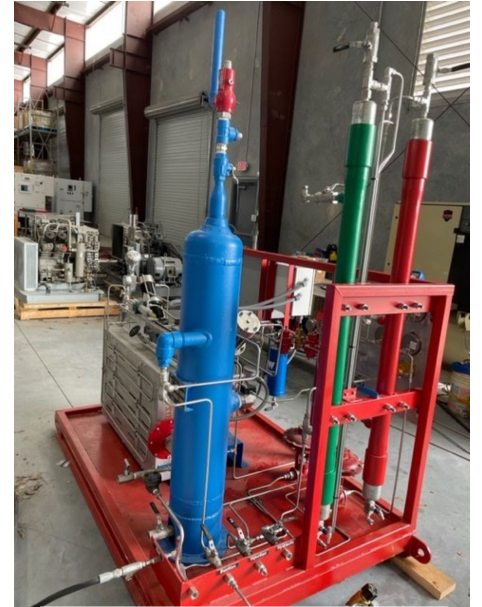
Gas Pump 10 HP Surface Control Skid
