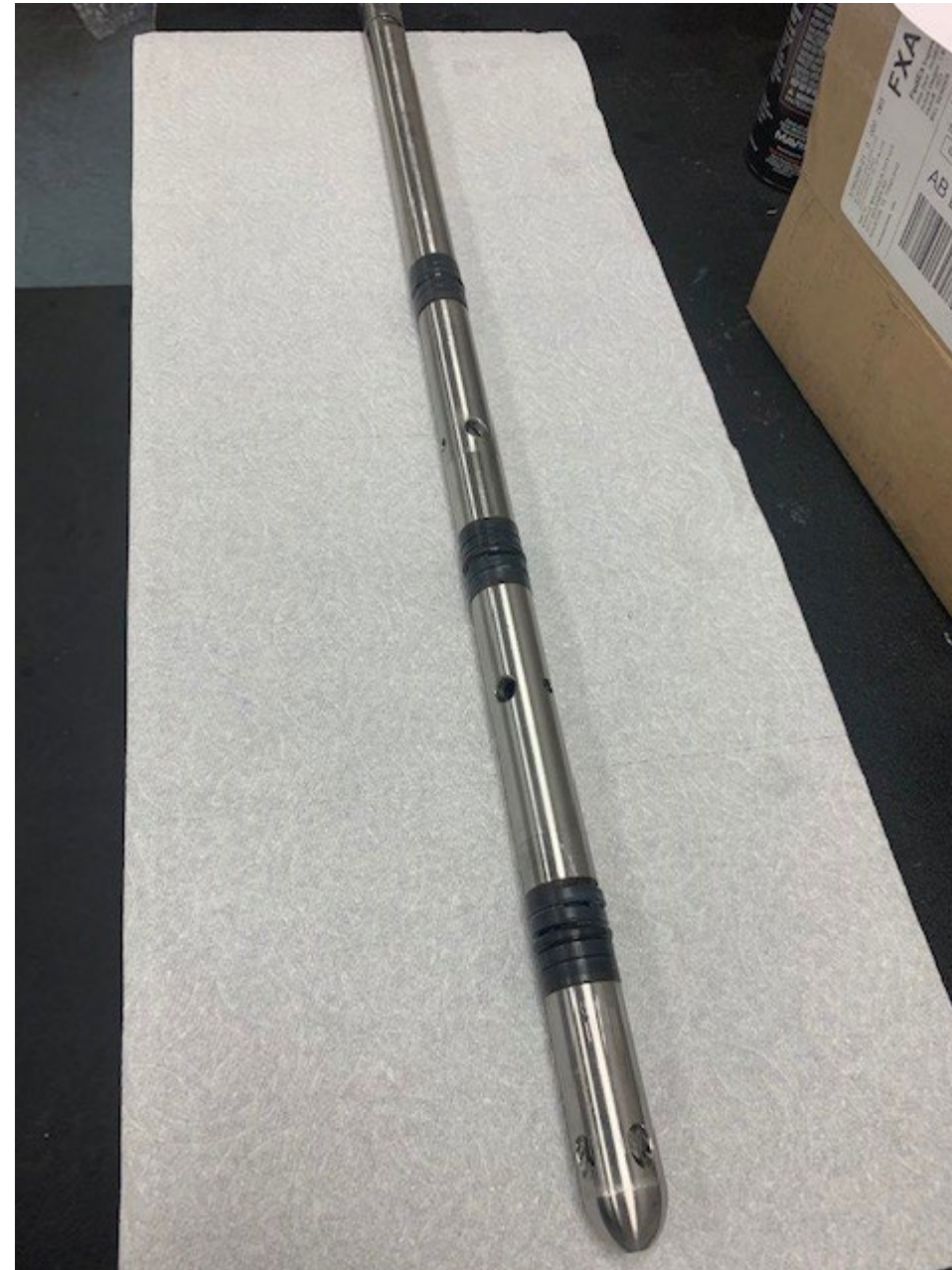
Gas Pump Injection Valve
