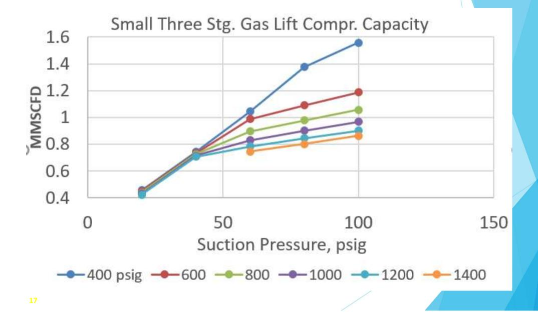
As wells mature, disparate injection pressures/ failure to change compressor operations can result in added costs and operational problems
